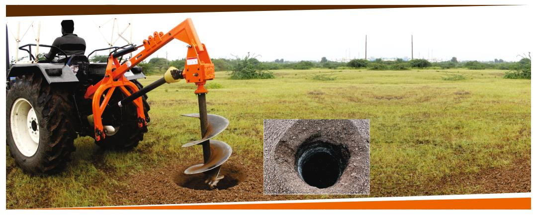
**SHAKTIMAN** Hydraulic Post Hole Digger (PHD) is tractor operated equipment to dig pits in agriculture or any other land with less time and effort. Manual digging pits is expensive, laborious and time consuming particularly when required to dig holes in mass numbers.
